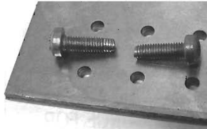
300 (18-8) stainless steel thread rolling screw with collapsed threads after trying to drive into a steel test plate (left) and a screw from the same lot before driving (right)
