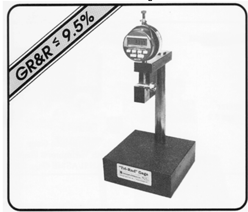
"Tri-Rnd" Gage for Measuring TAPTITE® Screws Patent #5,165,176
