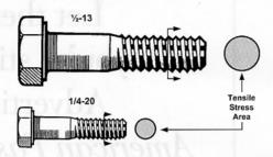
Fasteners with larger threads have larger tensile stress areas than those having smaller threads; therefore those within a given grade or strength class with larger threads can hold more weight before breaking (see Table 1).
