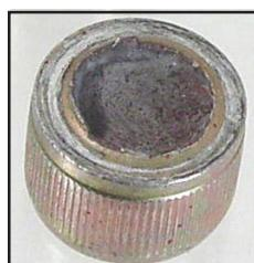
There are several classic indicators of a real hydrogen embrittlement failure. If any of these factors are missing, then the failure must be attributable to something other than hydrogen embrittlement. These five characteristics are:
