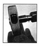
Step #6. Adjust the setting screw until there is a very light rotational resistance between the ring and the setting plug.
