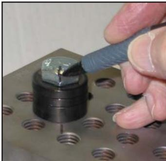
ii. Using a permanent marker, draw a mark on a corner of the bolt or nut. Mark a line out onto the surface of the application which lines up with the center of the bolt head and the marked corner.
