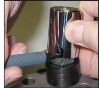
vi. Run the bolt or nut down close to the application surface and then place the socket which is on the torque wrench on the part so that the mark on the outside of the socket matches the marked corner on the fastener.
