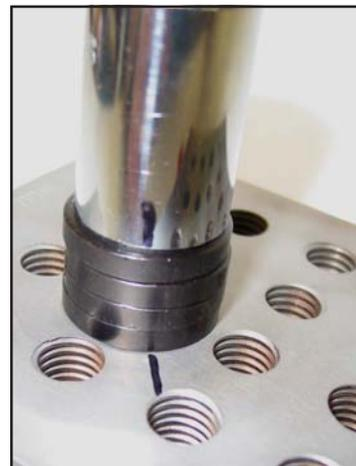
Apply torque with the torque wrench until the line on the outside of the socket lines up with the line you marked on the surface of the application before loosening the bolt or nut.
